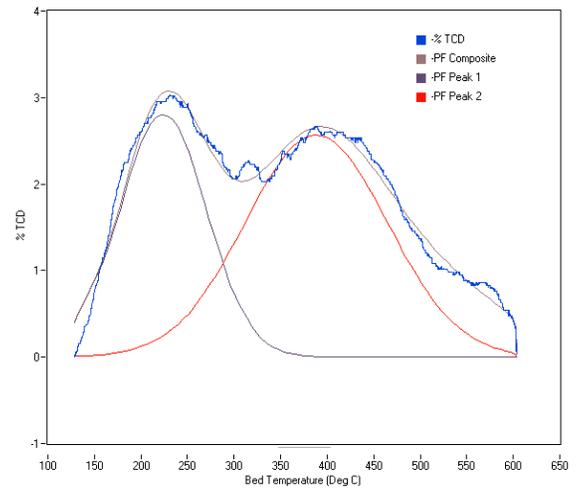
**Figure 5.** Peak deconvolution curves of ammonia TPD for the 125°C desorption
