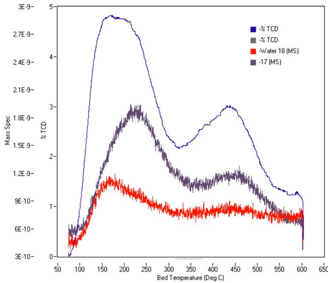
**Figure 4:** Mass spectral data during the TPD step for 75°C ammonia adsorption
