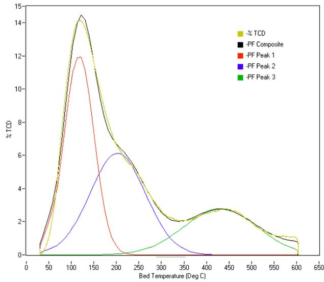
**Figure 1:** Peak deconvolution curves of the ammonia TPD for the 30°C adsorption
