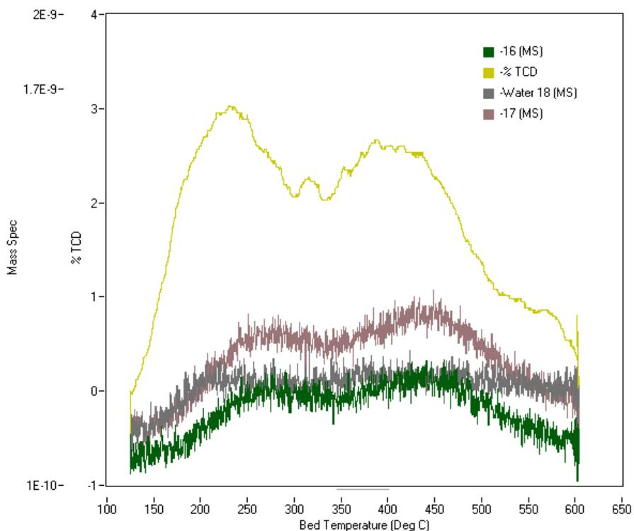
**Figure 6:** Mass spectral data during the TPD step for 125°C ammonia adsorption
