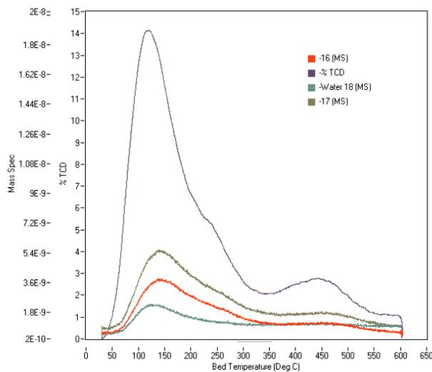
**Figure 2:** Mass spectral data during the TPD step for 30°C ammonia adsorption
