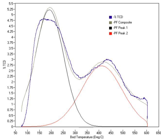
**Figure 3:** Peak deconvolution curves of ammonia TPD for the 75°C adsorption
