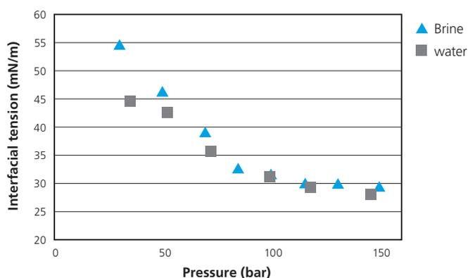
[Figure 2] Interfacial tensions between brine/CO<sub>2</sub> (triangles) and water/CO<sub>2</sub> (squares) as a function of pressure.
