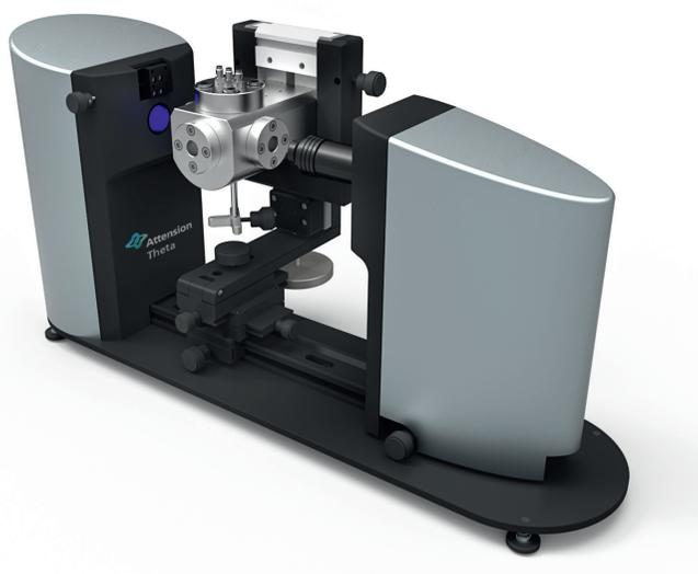
[Figure 1] Attension Theta with High Pressure Chamber.
