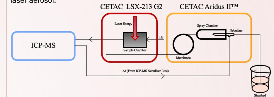
To obtain the liquid only signal, the ICP-MS was triggered and the laser shutter remained closed for 30 seconds. The shutter was then opened and a line scan (at 10 µm sec<sup>-1</sup>) was ablated for a further 30 seconds.
